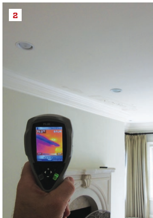
Water damage is evident on a ceiling above a second-floor fireplace (1). Infrared imaging confirms that the area is wet after rainstorms (2).
